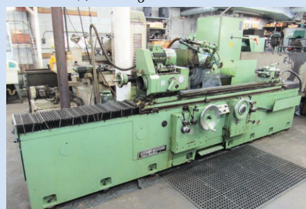
Kikinda Type C12 1600 14" x 63" Universal Cylindrical Grinder
